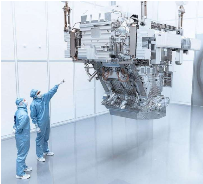
Figure 11: A German Zeiss lens for an ASML EUV lithography machine (Zeiss 2025)
