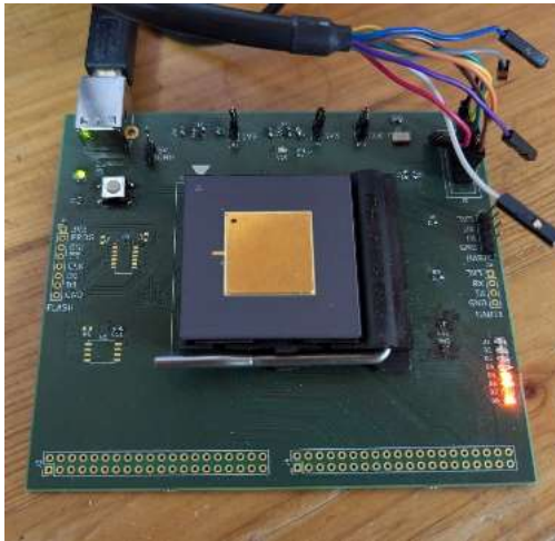
Figure 7: Prototype of an automotive Electronic Control Unit (ECU), to replace several other ECUs, designed with open tools (British/Spanish ChipFlow 2025a).
